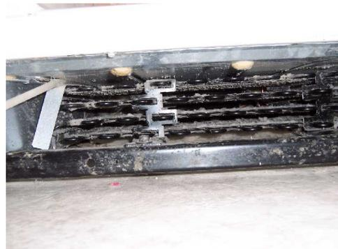
The dust that has collected inside the coils and around the compressor is what the start relay went out. The compressor will run to warm when it can not get enough air around the coils to cool itself.
