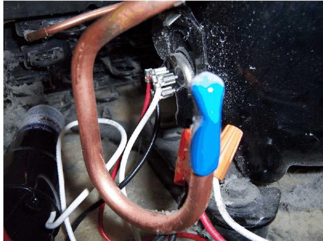
Above is a example of a compressor that has the terminals upside down from what is shown on the wire diagram that is on the 3n1 universal start relay.
