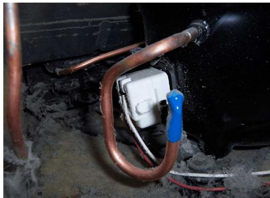
Remove the old start relay by pulling it off by hand. If it does not pull off by hand easily you may have to put the tip of a flat blade screw driver between the start relay and the body of the compressor to help pry it off. Most of the time you can remove them without any force.
