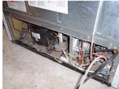
Once you have the back cover removed you will be able to see the compressor. The start relay will be located on the side of the compressor. The start relay shown on this side-by-side whirlpool refrigerator is white and has a white and red wire going to it.
