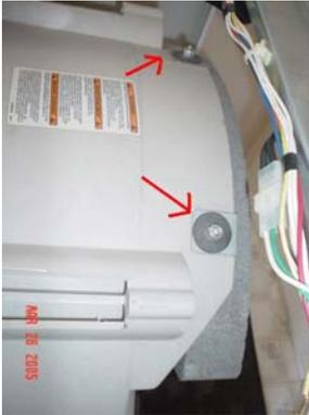
3. Remove drive belt. Cut zip tie, unplug motor and leave wiring in the bottom of the washer. Remove 4 screws that hold on motor and remove motor.
