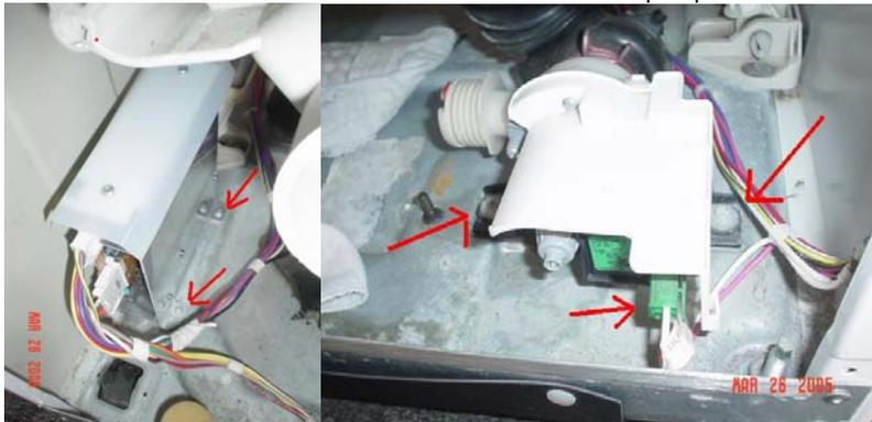
5. On shocks, push one lock area to allow the pint to be slid out of the tub and the shock will be free from the drum. Push pins through to the rear and remove. Will now be hanging from the springs.
