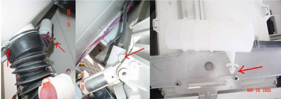
4a. At this point, you might want to remove the control board and pump motor. Each is secured by 2 screws and are easily removed. This will prevent accidental damage and give you more room inside the washer to work with. There are 2 connectors on the control board and 1 on the pump motor – be sure to remove those first.
