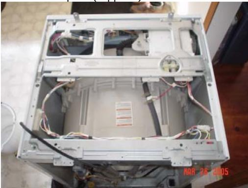
9. From above, lift drum and slide out the rear.
