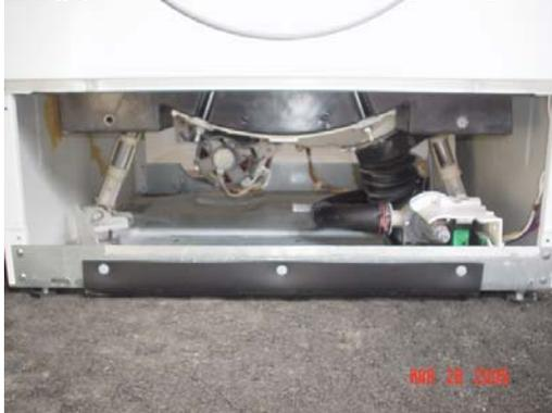
18. Move springs to correct holes on top. Install safety clips back over springs.
