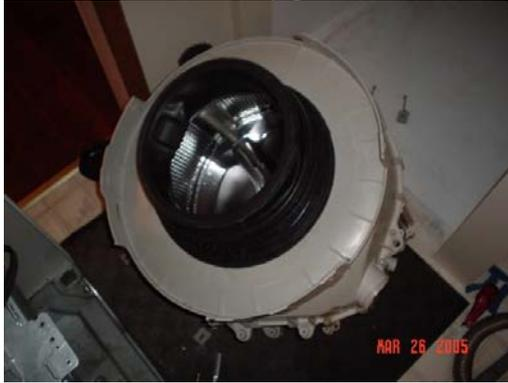
14. Without spring in boot, line up UP pointer and re-install boot to drum. Then pull spring back into groove on boot.
