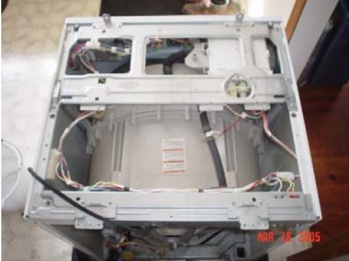
2. Loosen two screws that hold weight on back half and slide out weight. Leave screw on drum
