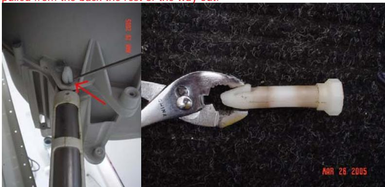
6. From top, slide out what looks like overflow tube from holder. Leave tube attached to the drum. Place support under drum. I used 2 5 qt. Ice cream pails, but they may be a bit light for the job.
