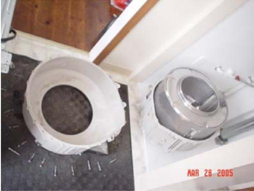
11. Remove and replace tub seal. New seal is thicker than old one....
